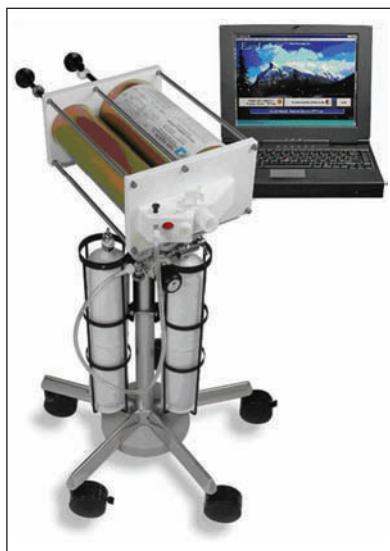
Figure 3. Gas transfer test simulator.
